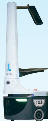
Locus is designed to function as the projector on wheel, an idea different from Kiva robots which is designed to lift the specially-designed shelf. In addition, Locus can lift bin on tray / tote and they are equipped with a scanner to avoid obstacles.
